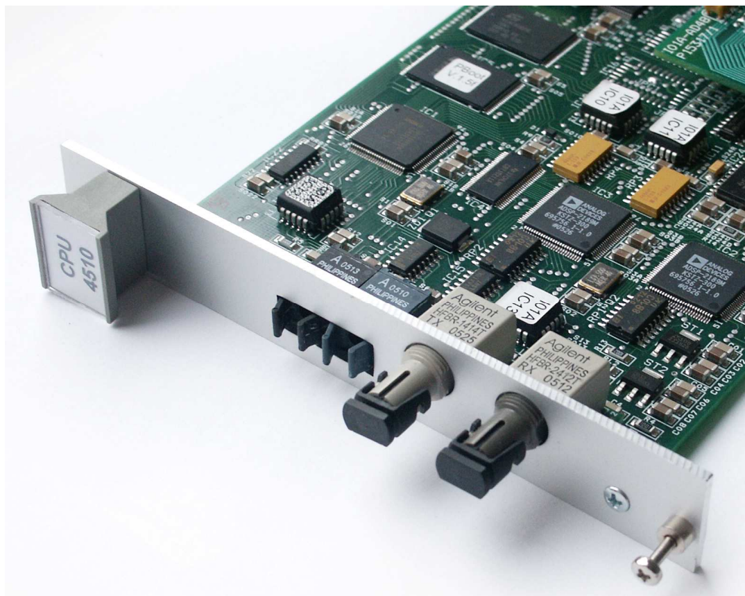
Multimode glass fibre optic cable connection
